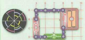
Make a paper disc with lines on it like the one shown here (a sample for cutout is on page 46 of project manual #1). Tape it to the fan blade and place it on the motor. Place this circuit under a white fluorescent light in your home or school (don't use an ordinary incandescent lamp). As the speed changes you will notice the white lines first seem to move in one direction then they start moving in another direction.
