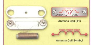
The antenna you will use is a  $25\mu H$  coil wrapped around an iron bar, which increases the inductance to  $300\mu H$ . Although it has magnetic effects similar to those in the motor, those effects are tiny and may be ignored except at high frequencies (like in AM radio). At low frequencies the antenna acts like an ordinary wire.
