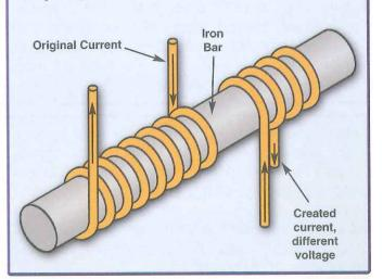
Important Note: Transformers only work with changing voltages (AC). Unchanging voltages (DC) have no magnetic properties and don't work with transformers. Many motors (like the one in snap circuits) have a mechanical design that allows them to use the DC voltage from batteries.
