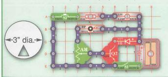
Using the fan outline as a guide cut a 3" circle out of a piece of paper. Then, cut a small triangle in it as shown. Tape the circle onto the fan and then place it onto the motor. Set the adjustable resistor to the center position and turn on the switches. The fan spins and the lamp lights. As the triangle opening moves over the photoresistor, more light strikes it. The brightness of the LED changes, or is modulated.
